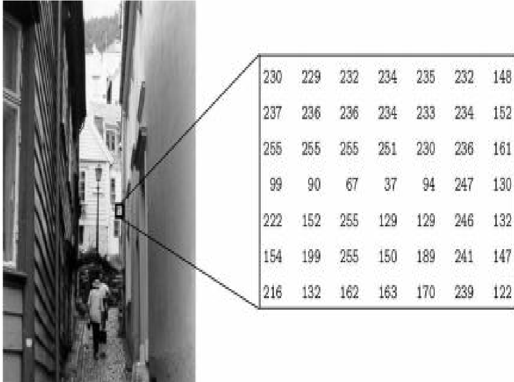
Figure 2.1: Grayscale image and its one minor part representation as rows and columns of numbers.
