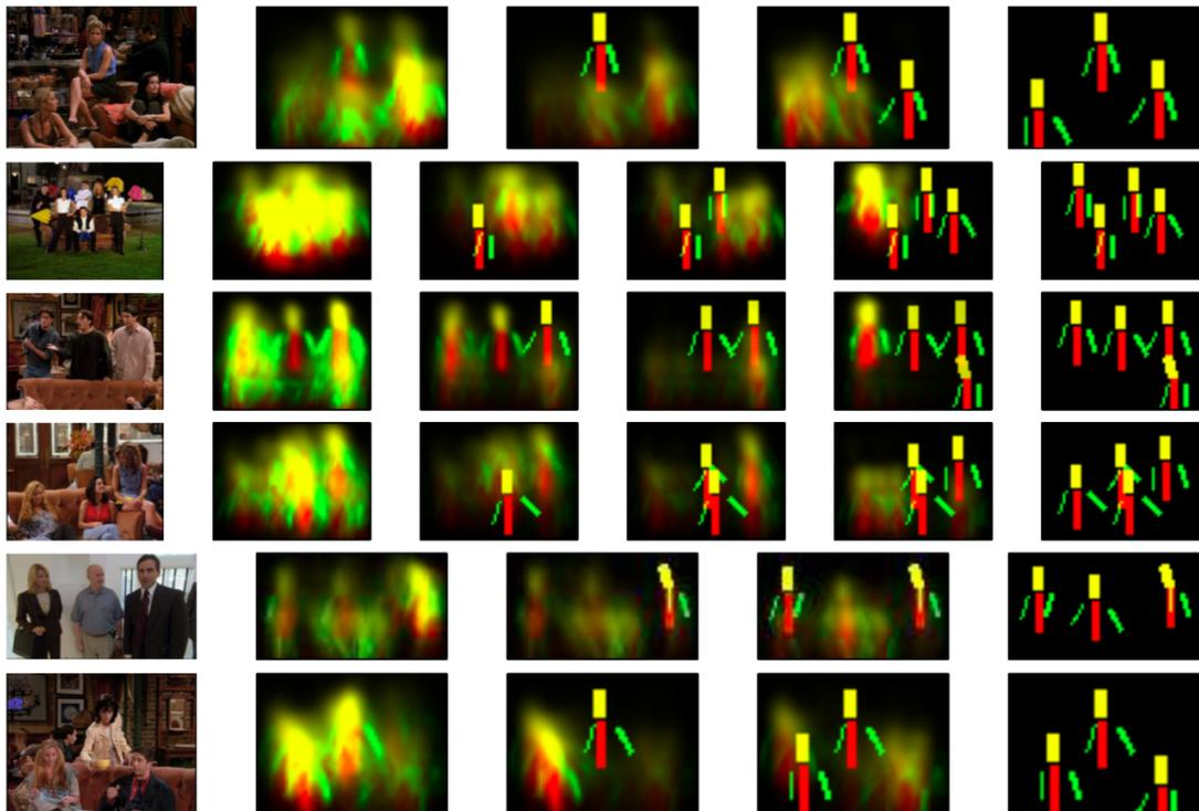
Figure 0.1: The successive selection of poses in a picture using a DPP based on the quality of the poses which is depicted in the second column. Original graphic due to [KT10].
