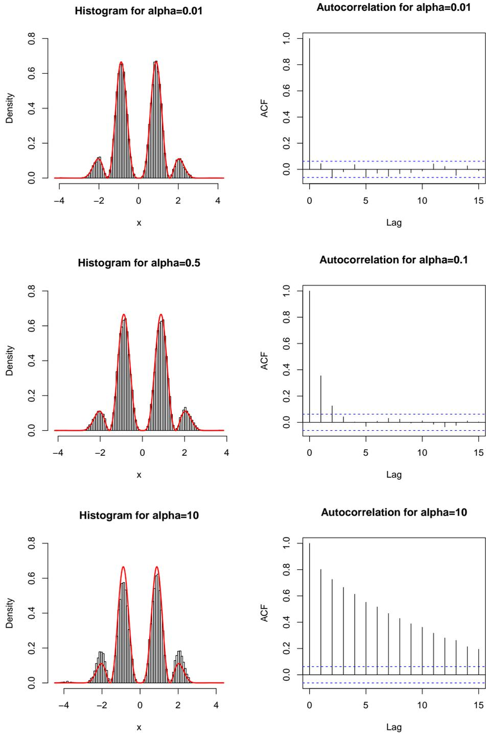
Figure 3.4: Histograms and autocorrelation functions for the choices of  $\alpha = 0.01, 0.5, 10$ . The auto correlation obviously decreases the fastest for  $\alpha = 0.01$ , however the computation time is much higher than for the parameter the other parameters.
